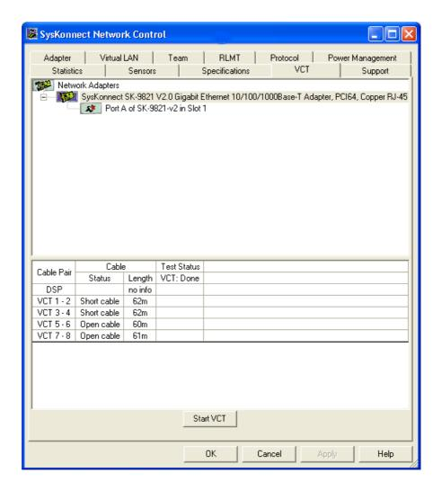
Figure 4. Display after a VCT test
